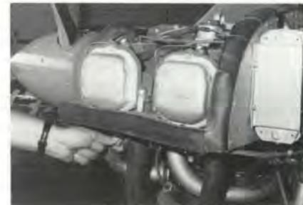
Mounted behind the engine, there's little you can do to check this magneto until the check at the end of the runway. It's a check you don't want to skip.
