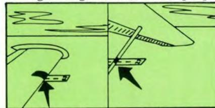
er pattern altitude, and with the wings level, the aircraft will be at the correct distance from the run-
