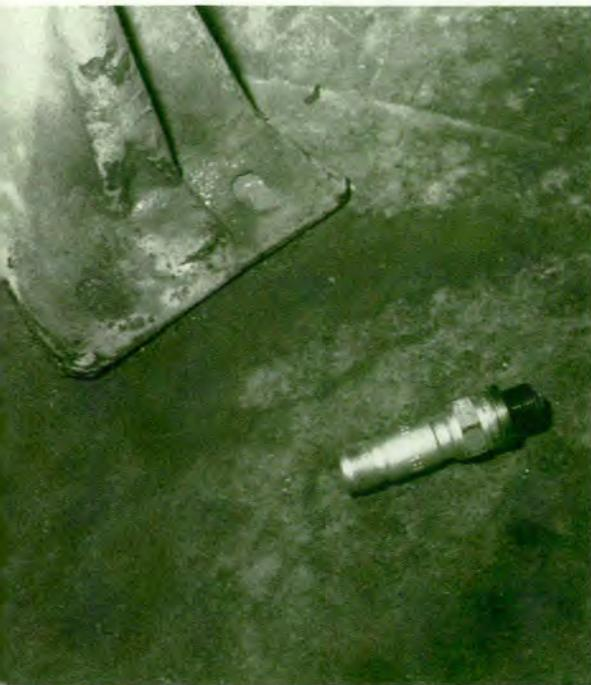
"If you drop it once, drop it again — into the trash." Trying to see a crack in the insulator of the spark plug below is virtually impossible. Cracked insulators are sure to fail at the worst possible moment.
